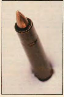
7.62x62.8mm cartridge case is beveled at the mouth and 2.46mm thick in this area to withstand the radial stresses which occur at the internal stop shoulder when it is impacted by the piston within the case. Photo: Peter G. Kokalis
